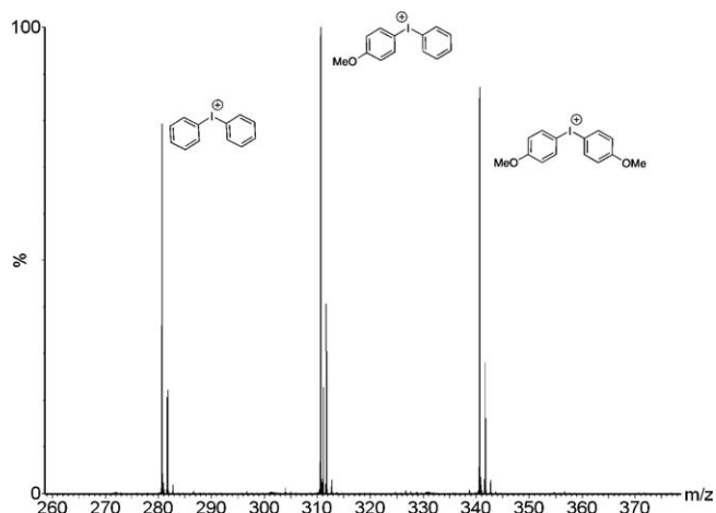
Fig. 6. ES-MS spectrum of 1(OTf) after it had been treated with TMAF followed by TMSOTf.
